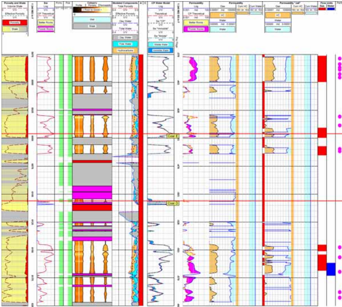
Figure 10: Examples of Capillary Pressure/Petrophysical Modeling – MV 4-3 well.
